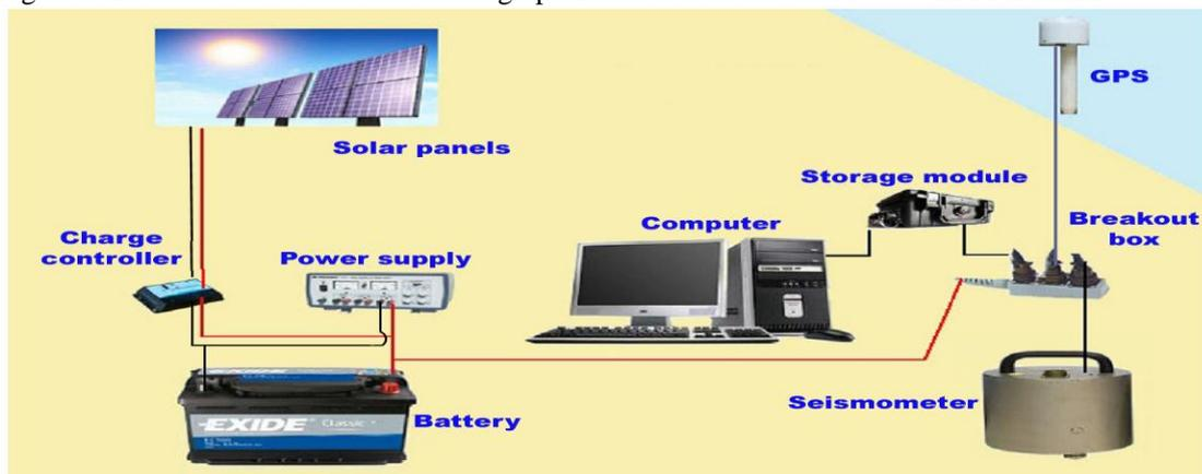
figure 2. Block diagram of educational seismograph setup
