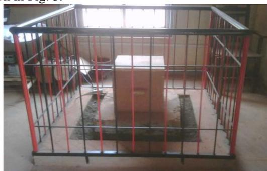
Figure 3. Seismometer pit with the broad-band seismograph covered with an insulated box
